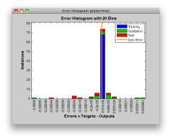
The dynamic response can be plotted, with colors indicating how targets were assigned to training, validation and test sets across timesteps. (Dividing data by timesteps and other criteria, in addition to by sample, is a new feature described in "New Time Series Validation" on page 13-9.)
